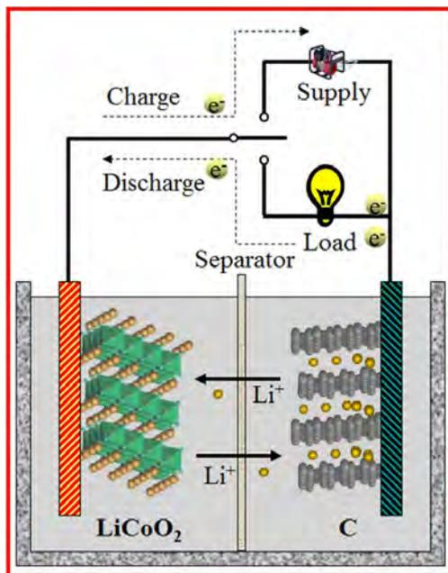
**Figure 2** - Schematic diagram of the fundamental structure of Li-ion batteries. The anode is carbon, and the cathode is  $\text{LiCoO}_2$  in this image. [Energy Science and Engineering, 2015, 3, 385]
